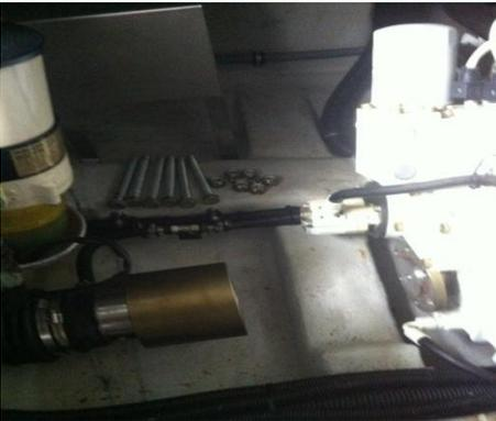
4. Unscrew the rubber shaft seal with the graphite ring
