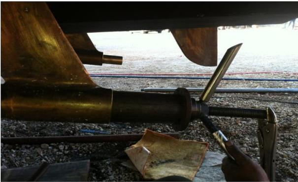
8. Carefully clean the bearing beds and grind with fine sand paper on the surface
